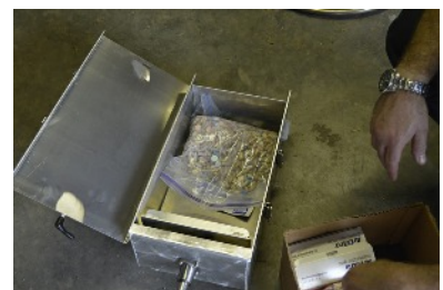
Step 3: Drugs are put into the incinerator's injector box.
